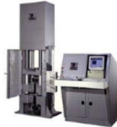
Fig. 4.4.5f A High Capacity UTM for Testing Ultra High Strength Concrete Cylinders
