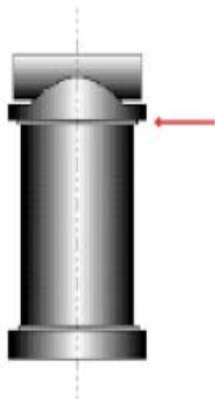
Fig 4.4.5d Spherical Platen ensures that the load is transferred evenly to the Concrete Cylinder
