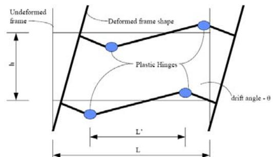
Figure 7-1 - Desired Plastic Frame Behavior
