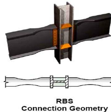
The RBS or “*Reduced Beam Section*” also known as the “*Dog Bone*” because of its shape introduces a weakening at the Beam or girder to allow it to fail in ductile mode ahead of the column.
