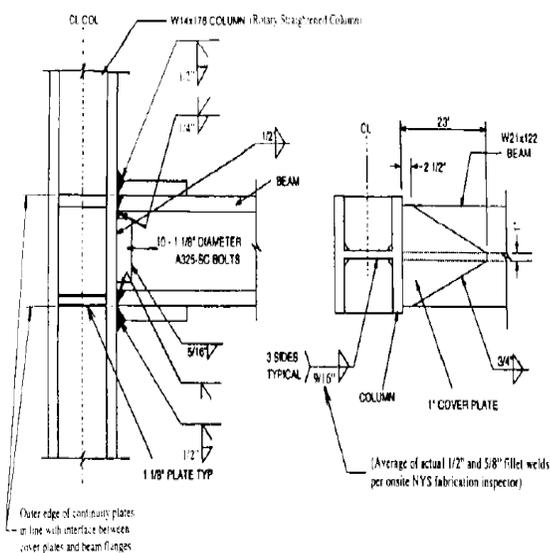
Figure 4 Revised Type 3 Connection
