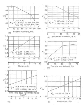
Figure 2-7 Shrinkage correction factors for the ACI 209 method of shrinkage prediction. Note that at standard conditions K\*=0
