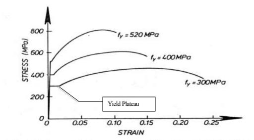
Typical stress-strain curves for reinforcing steel. (1 MPa = 145 psi.)
