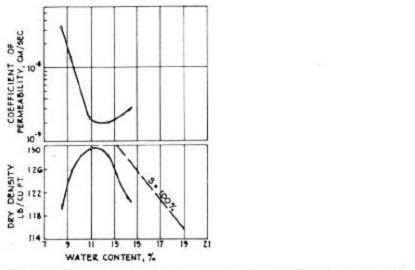
Figure 8.5 Effects of compaction water content on soil permeability. (After Lambe, 1958.)
