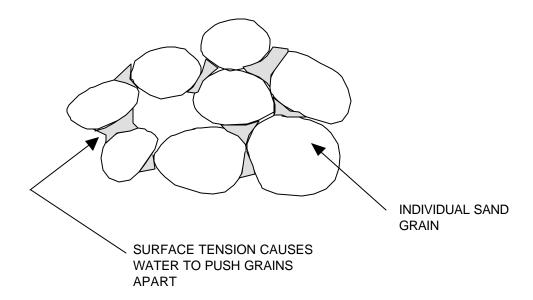
A very dry sand in the hand can not be squeezed into shape whereas a semi moist sand when squeezed could hold some shape until it dries out and crumbles. Surprisingly, addition of more water to saturate the sand collapses the sand as in the very dry state.
