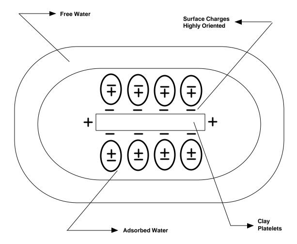
As we can see, the clay is composed of submicroscopic platelets surrounded by Electrical charges, a closely held layer of adsorbed water and an outer layer of
