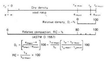
Figure 8.9 Relative compaction—relative density relationships. (After Lee and Singh, 9th Annual Engineering Geology and Soils Engineering Symposium, Boise, Idaho, 1971.)
